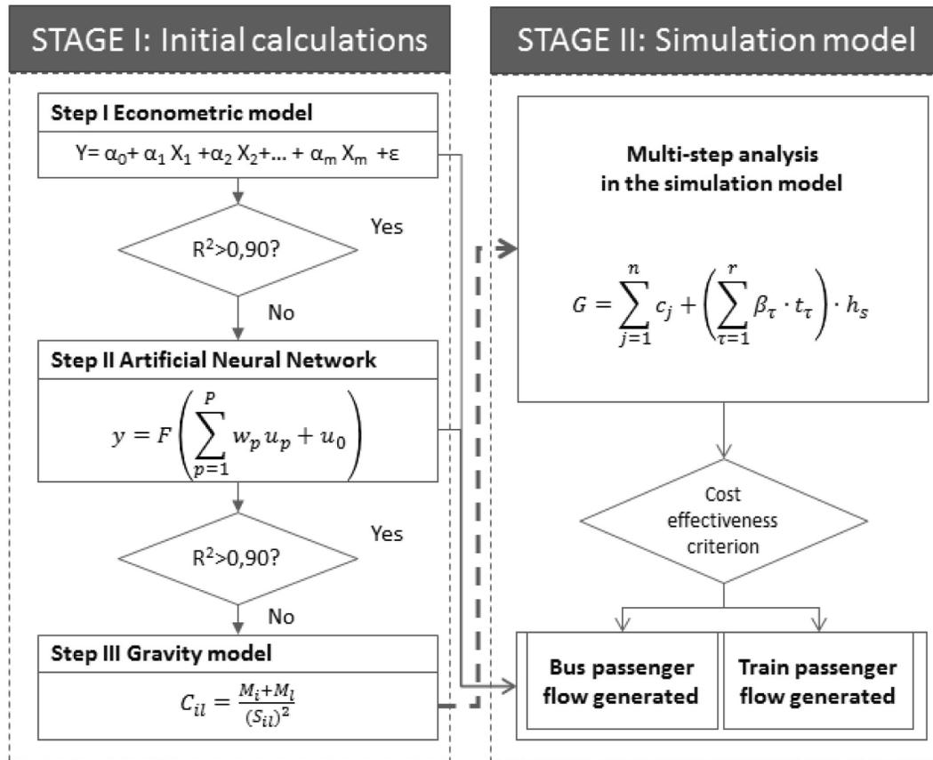
Fig. 1. The methodology used to develop a simulation, advising tool.
