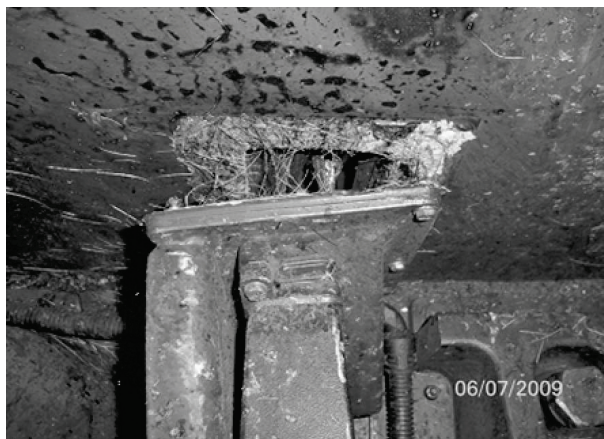
Fig. 5. The bottom of a driver's cabin floor after a collision with a big animal; a damaged Hasting's joint (photo: K. Wiśniewska)
