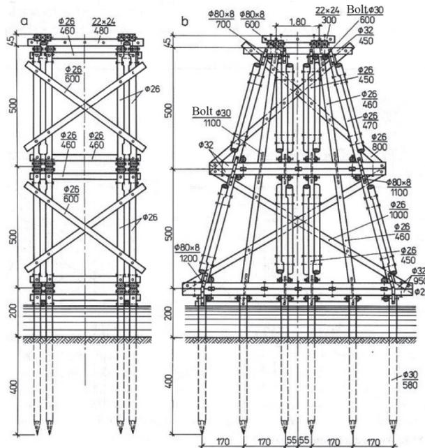
Fig. 5. Pillar made of two sets of piles, located symmetrically in relation to the longitudinal axis of the girders [3, 8]. Pillar height  $h = 10$  m;
