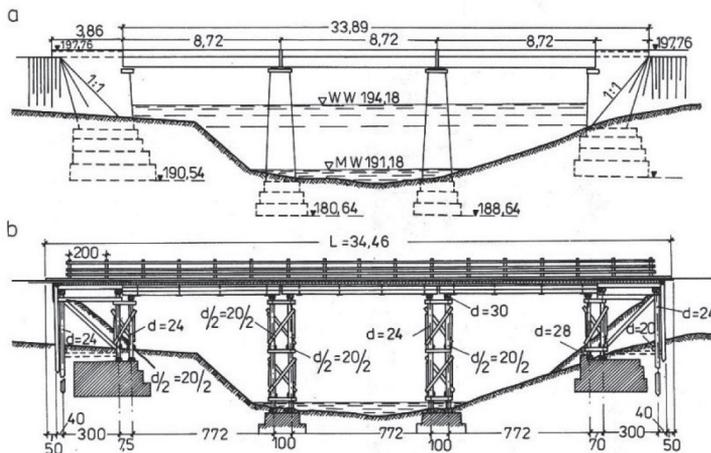
Fig. 13. Provisional reconstruction of the road bridge on frame supports [3, 8]: a - view of the bridge before destruction, b - provisionally rebuilt bridge
