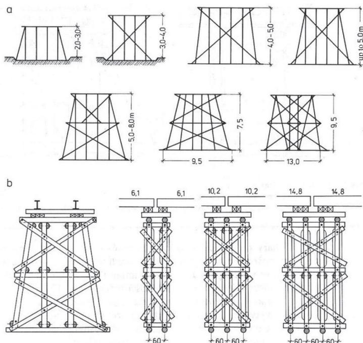
Fig. 8. Frame supports [3, 8]: a - cross-section diagrams of the bridge carriageway, b - support structure in the cross-section of the bridge carriageway and view of the supports (two-row, three-row and four-row) in the longitudinal direction of the bridge spans
