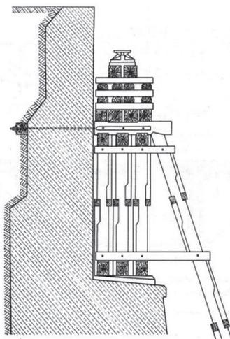
Fig. 14. The structure of the frame support in the abutment niche, attached with steel anchors to the abutment wall [3, 8]
