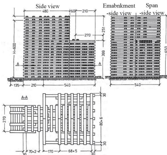
Fig. 4. Bridge abutment, constructed of cages composed of railway sleepers [3, 8].
