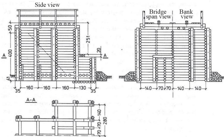
Fig. 11. Cribwork abutment [3, 8]: upper left - side view (along the bridge span), upper right - front view (in the cross-section of the bridge span), bottom left - horizontal A-A section
