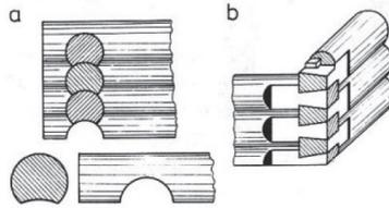
Fig. 10. Connection of corners in cribwork [3, 8]: a - normal connection, b - connection on rivers with high ice floe flow
