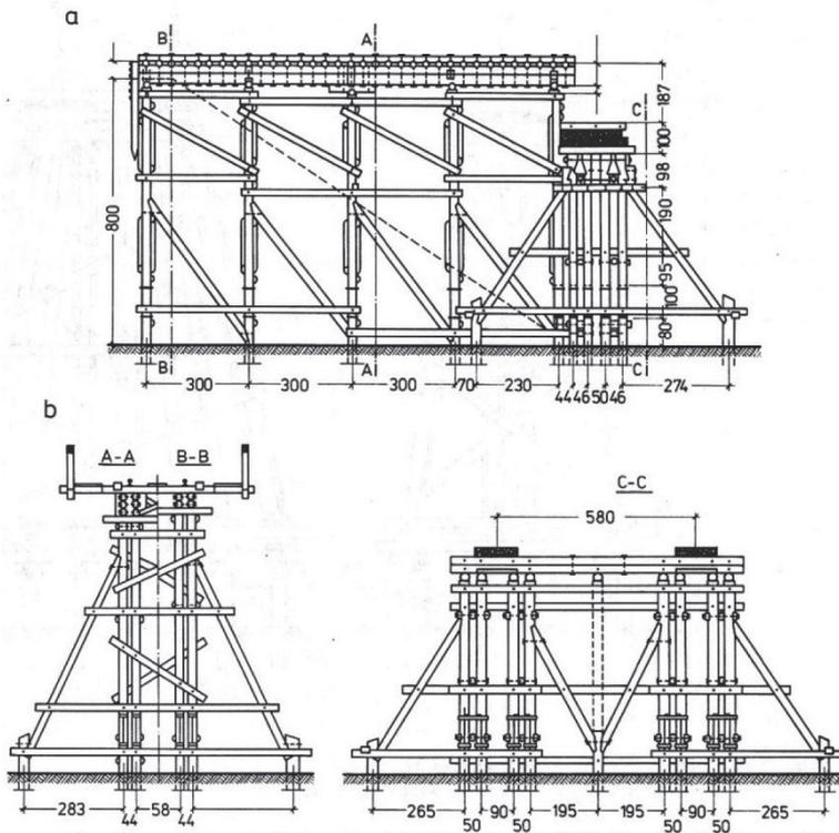
Fig. 7. Wooden abutment, consisting of two parts [3, 8]: a - longitudinal view, b - cross sections of the abutment A-A and B-B, c - cross-section view of the support C-C bridge span
