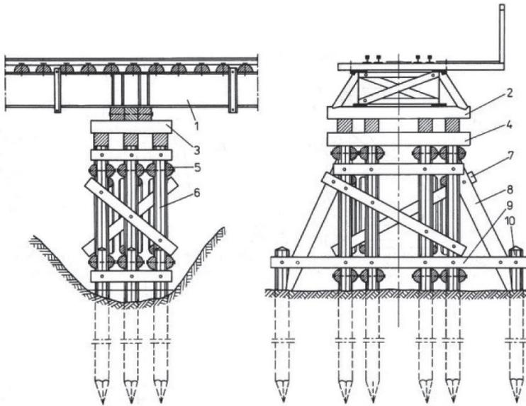
Fig. 6. Pillar of the provisional bridge [8]: left - in the longitudinal section through the bridge structure; right - in the cross section through the bridge structure; 1 – bridge span, 2 - bearings, 3 - beam substrate, 4 - cap, 5 - horizontal brace, 6 - main piles, 7 - oblique clamp, 8 - braces, 9 - horizontal clamps, 10 - strut piles
