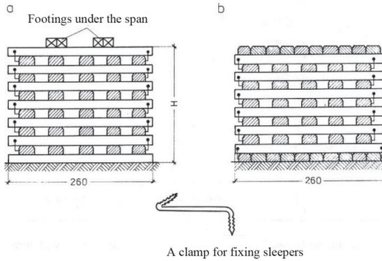
Fig. 1. Cage made of wooden railway sleepers [8]: a - side view (longitudinal direction of the bridge spans, b - front view (in the cross-section of the bridge span)
