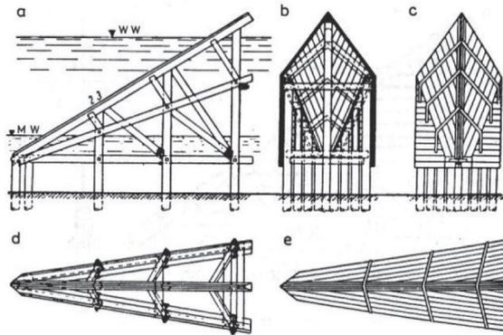
Fig. 16. Tent ice aprons [3, 8]: a - side view of the ice apron frame (without formwork), b - rear view (in the direction opposite to the water current vector), c - front view (in the direction of the water current vector), d - top view of the ice apron frame, e - top view of the ice apron with formwork
