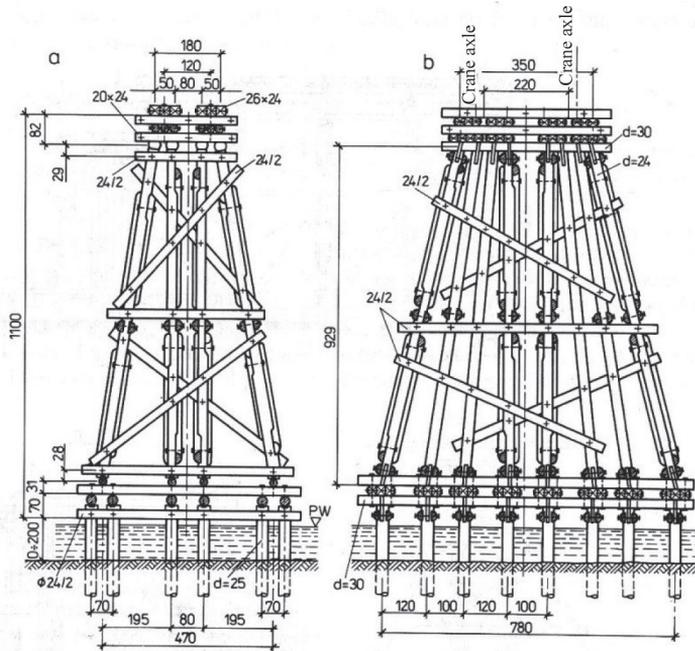
Fig. 9. Frame-pile support 11.0 m high [3, 8]: a - side view of the pillar (in the longitudinal direction of the bridge spans), b - front view of the pillar (in the cross-section of the road set on two main girders)
