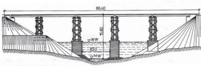
Fig. 12. Cribwork-frame supports [3, 8]
