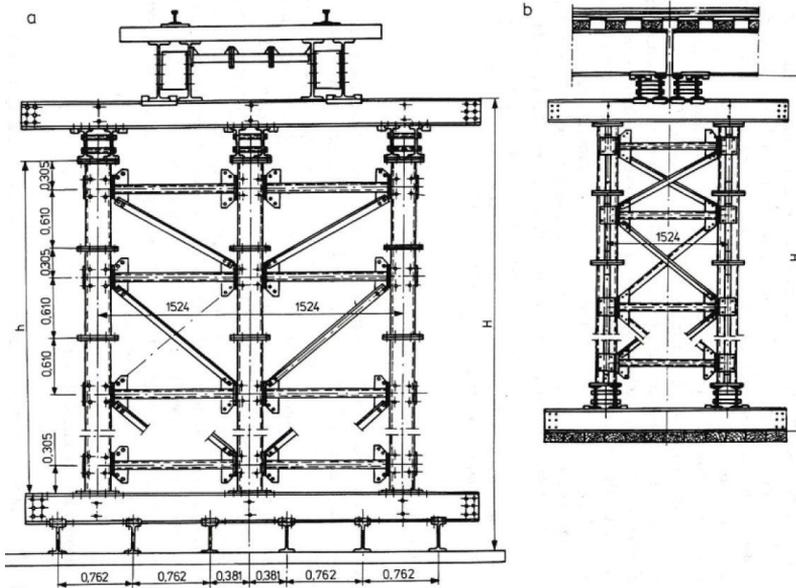
Fig. 18. Collapsible frame support (pillar) of a railway bridge on a single track line [8]: a - view of the pillar in the cross-section of the bridge span, b - pillar in the longitudinal view of the bridge spans
