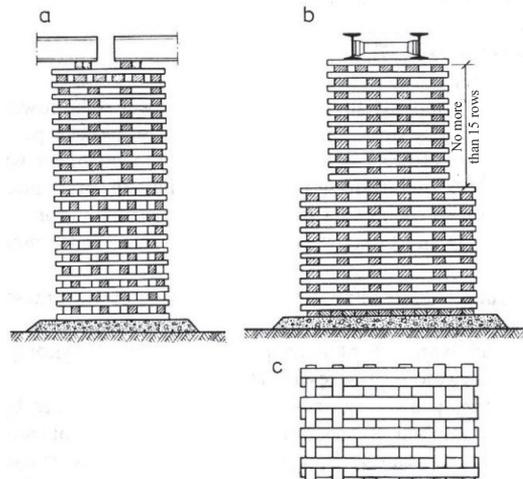
Fig. 2. Bridge pillar constructed of cages composed of railway sleepers [3, 8]:
