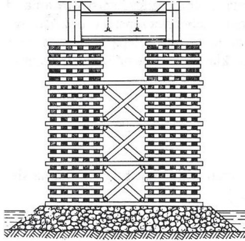
Fig. 3. Cross-section through the bridge span on a pillar constructed of two sets of cages composed of railway sleepers [3, 8]
