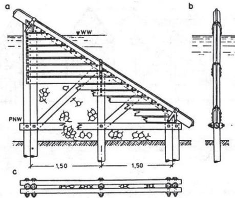
Fig. 15. Single ice apron [3, 8]: a - side view (in the plane of the vertical cross-section of the bridge span), b - front view (along the bridge span), c - top view
