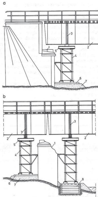
Fig. 17. Schemes of structural systems of the steel folding support [8]: a - folded support in the process of reconstructing the abutment, b - folding supports during the pillar reconstruction; 1 - damaged support elements, 2 - ends of the bridge spans (in the longitudinal view), 3 - reinforcement of the webs of the main beams in the bridge spans, 4 - support bearing element, 5 - cap elements, 6 - support elements, 7 - direct foundation (a layer of stone aggregate), 8 - wooden cribwork
