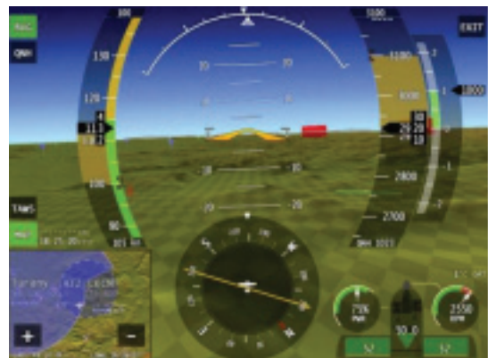
Fig.7. Display of the ground test control station
