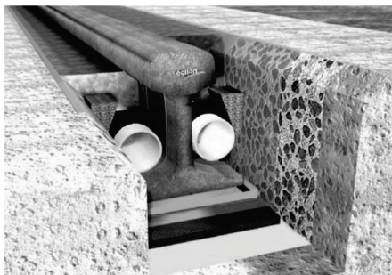
Fig. 10. Cross-section of ERS pavement as well as components and the construction process.
