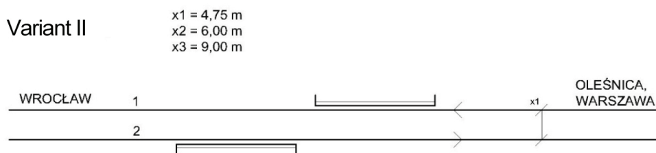
Fig. 3. Variant II of the track layout of the passenger stop. Source: own study.
