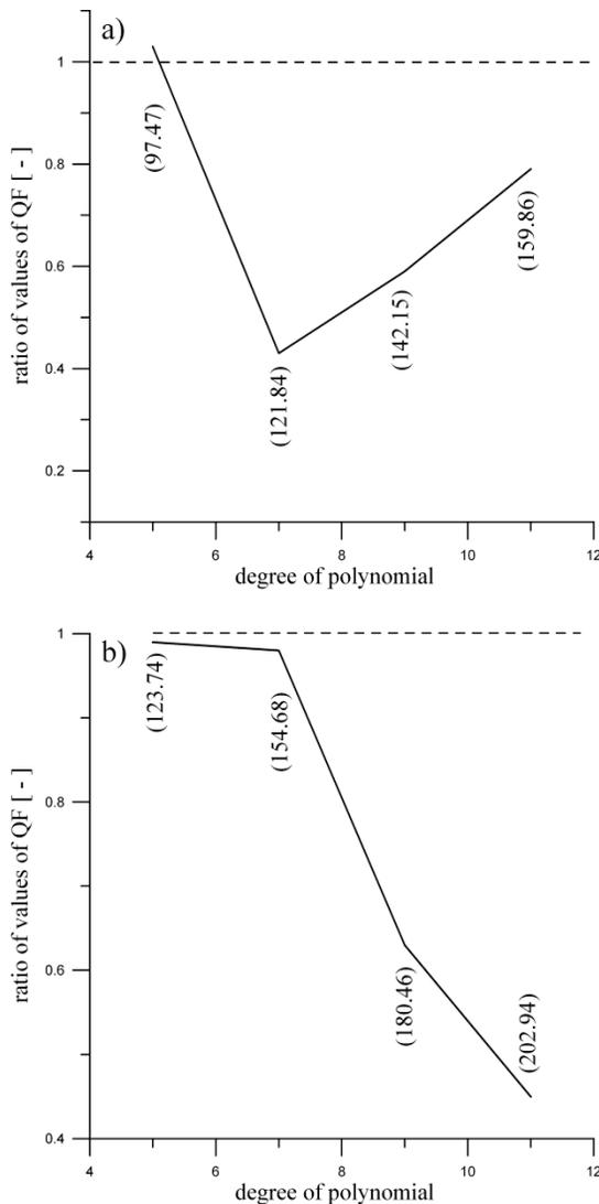
Figure 5.5 Comparison of ratio of values of QF for optimum TCs with maximum number of terms to value for 3<sup>rd</sup> degree parabola: a) v=24.26 m/s, b) v=30.79 m/s. Values in brackets are lengths of TCs
