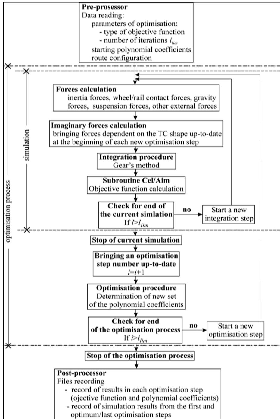
Fig. 4.1. General scheme of the software to optimise transition curves' shape.
