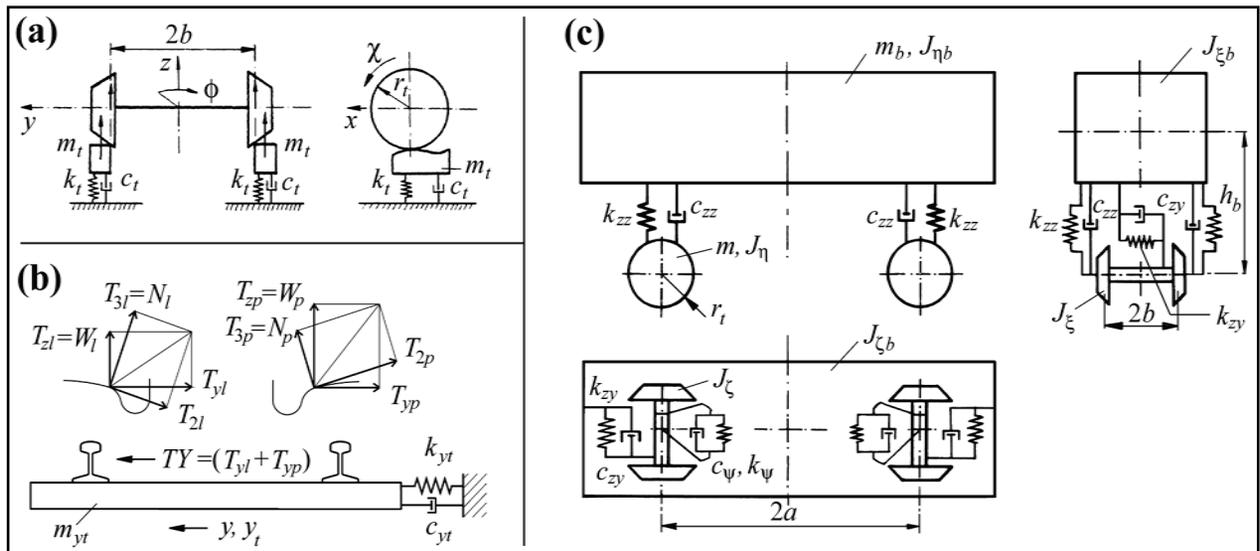
Fig. 3.1. System's nominal model: (a) track vertically, (b) track laterally, (c) vehicle.
