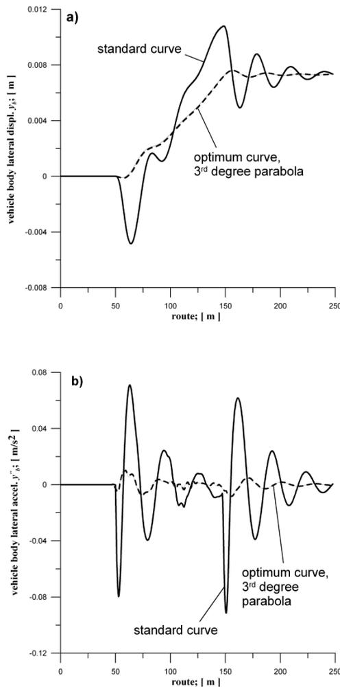
Fig. 5.2 Comparison lateral: a) displacements, b) accelerations of vehicle body
