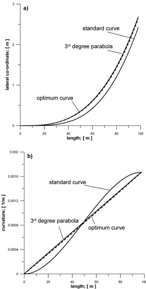
Fig. 5.1 Comparison: a) lateral co-ordinates, b) curvatures of transition curves – standard curve of 5<sup>th</sup> degree, the curve (5.1), and the 3<sup>rd</sup> degree parabola
