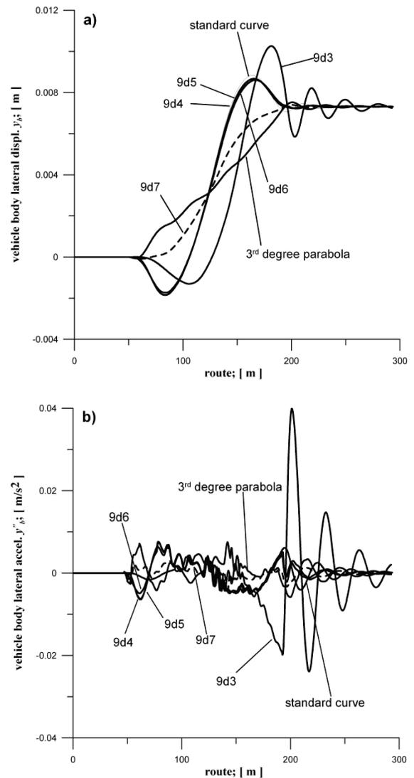
Fig. 5.4 Comparison of lateral: a) displacements, b) accelerations of the vehicle body for curves from Fig. 5.3
