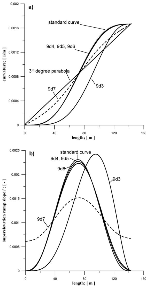
Fig. 5.3 Comparison of: a) curvatures, b) superelevation ramp slopes of transition curves of 9th degree with a different number of terms - 3, ..., 7, and 3rd degree parabola
