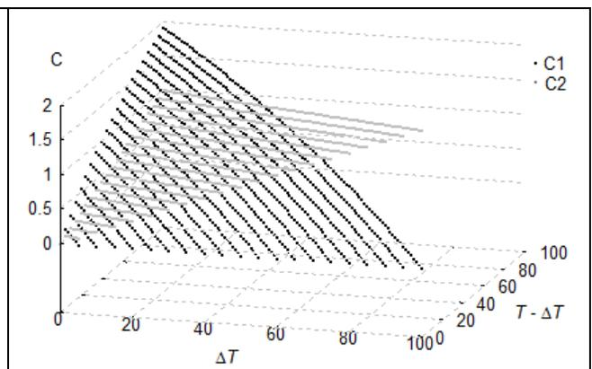
Figure 4. The costs of increasing unreliability (C1) and element’s rejuvenating (C2) when returned element is reused in a new production ( $C_R = (\Delta T + T) / 100$ )
