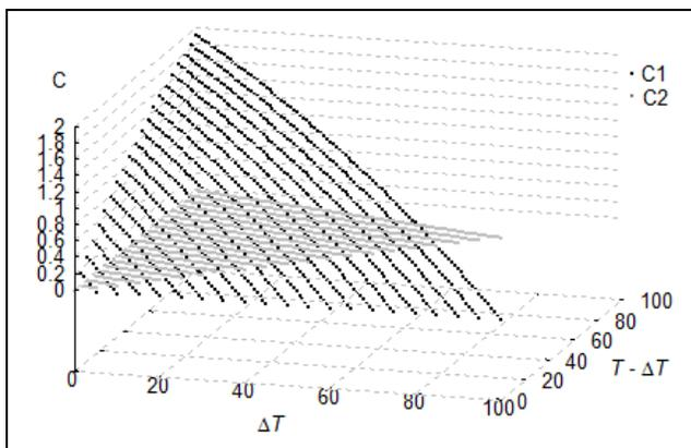
Figure 3. The costs of increasing unreliability (C1) and element’s rejuvenating (C2) when returned element is reused in a new production ( $C_R = \Delta T/100$ )
